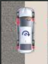
Braking control on a road surface with different left and right side traction characteristics
